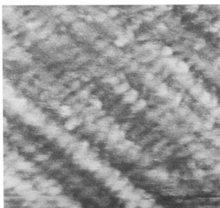
Fig. 4: LF nanograph of UHMW PE tape ( \lambda = 10 ), which shows nanofibrils with shish-kebab type structure. Area is 450 \times 450 \text{ nm}^2 . The meaning of gray-scale contrast is the same as in Fig. 3c.
